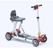
Motion Healthcare mLite Max weight capacity: 115kg Max speed: 4mph Max range\*: 9 miles
