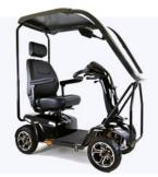
One Rehab Komfi Rider Alpine with Solid Canopy Max weight capacity: 181kg Max speed: 8mph Max range\*: 35 miles
