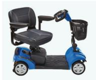
**Electric Mobility Veo Sport LiFe** Max weight capacity: 130kg Max speed: 4mph Max range\*: 16.3 miles
