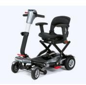
**TGA Minimo Autofold** Max weight capacity: 115kg Max speed: 4mph Max range\*: 10 miles
