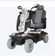
Kymco Maxi XLS Max weight capacity: 200kg Max speed: 8mph Max range\*: 35 miles
