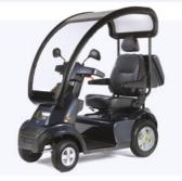
TGA Breeze S4 Long Range Battery & Solid Canopy inc Sides Max weight capacity: 200kg Max speed: 8mph Max range\*: 34 miles
